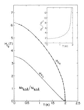
FIG. 1. Temperature dependence of the parallel  $H_{c\parallel}$  and perpendicular  $H_{c\perp}$  critical fields for Mo-Ni heterostructures with  $\lambda = 16.6$  Å. Inset shows critical field anisotropy. X-ray structural data indicate that layering is preserved in this structure.
