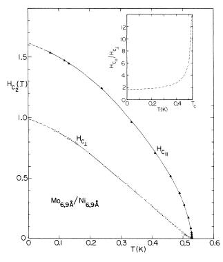
FIG. 2. Temperature dependence of the parallel  $H_{c\parallel}$  and perpendicular  $H_{c\perp}$  critical fields for structure with  $\lambda = 13.8$  Å. Inset shows critical field anisotropy. X-ray structural data reveal a typical glassylike diffraction pattern, signaling a structural collapse.
